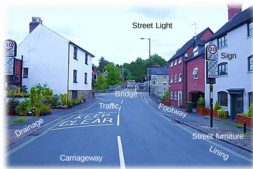
Figure 2. Types of Highway Infrastructure Assets
